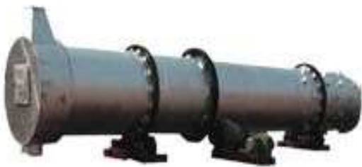
Rotary Drum Dryer
